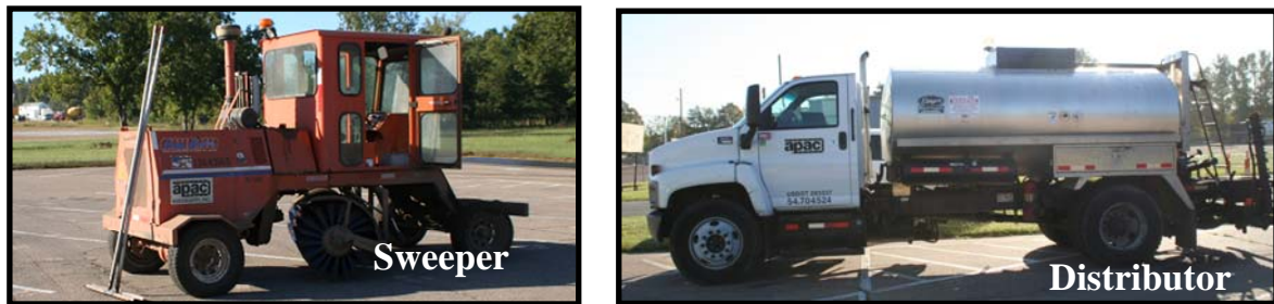
Figure 3.8. Sweeper and Tack Coat Distributor
