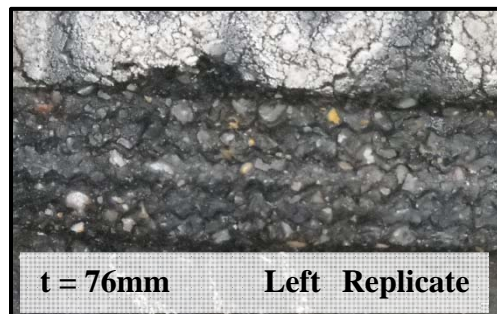
Figure A.23. PURWheel Wet Test Results for Strip 6
