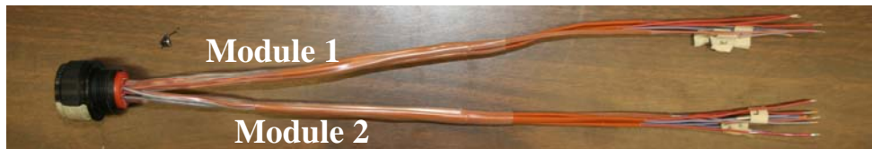
Figure 4.6. Male Connector (Trunk Line) and Stripped Ends (NI 9211 Modules)
