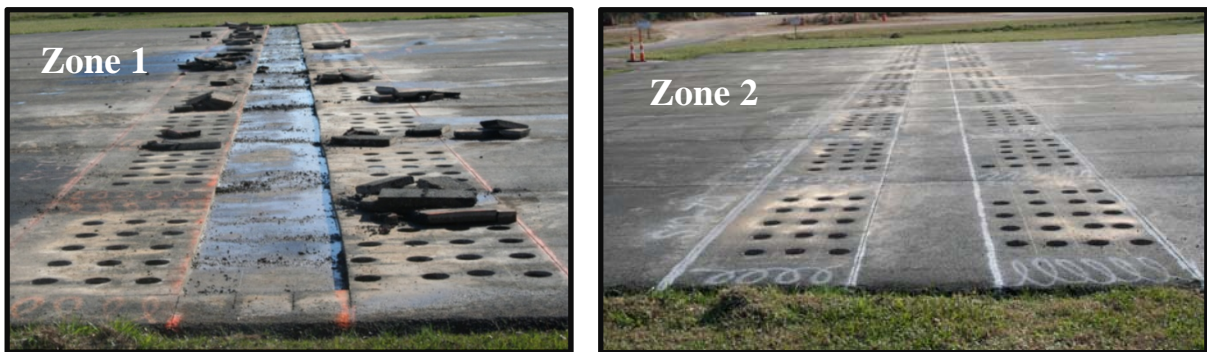
Figure 3.25. Test Zones at the Conclusion of Specimen Removal
