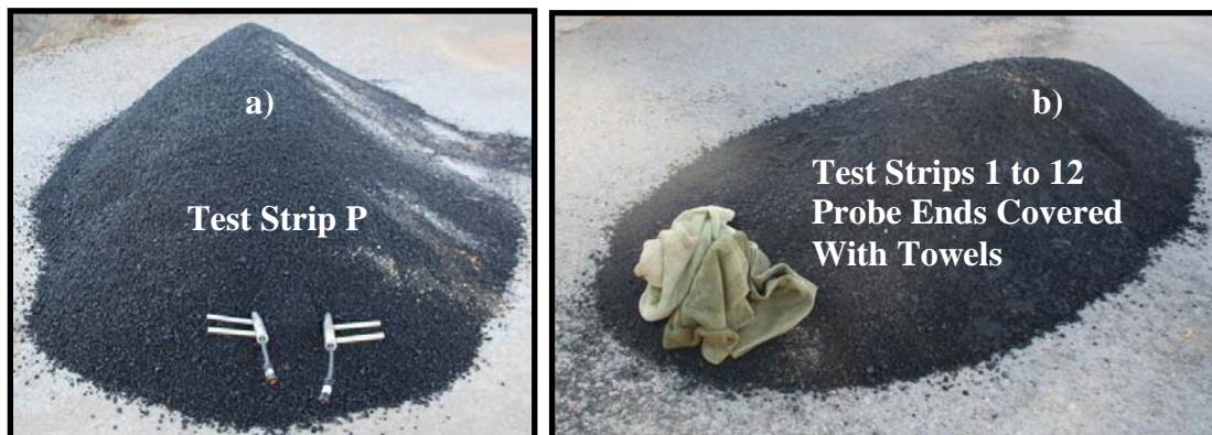
Figure 4.13. Pre-Heating Probes With Plant Mixed Asphalt
