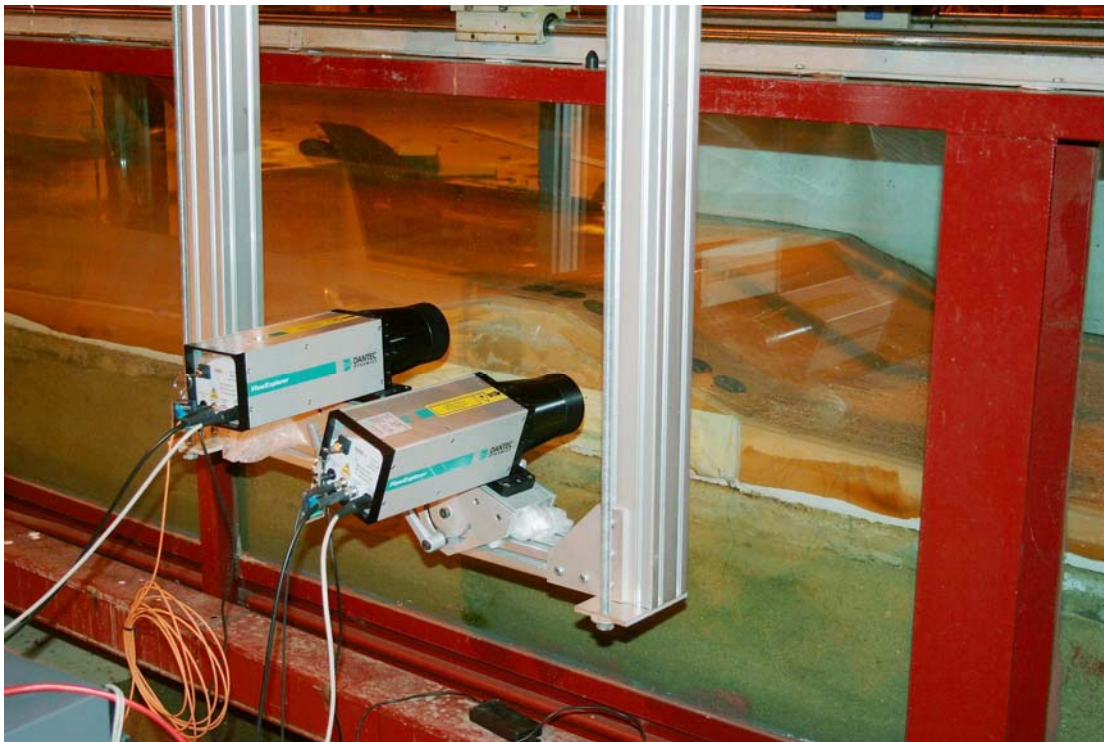
Figure 3.6. Laser Doppler velocimeters positioned outside the wave flume.
