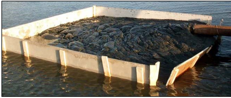
Figure 2.1. Wooden Box Testing of Dredged Material of Martin (2002) Provided by ISTC
