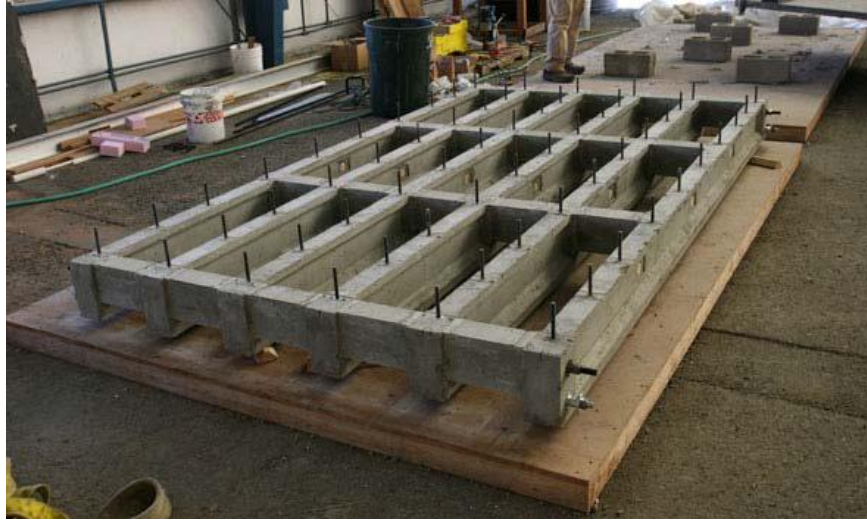
Figure 3.9. OSU Model of a typical Escambia Bay Bridge Section Over Escambia Bay (Bradner 2008).
