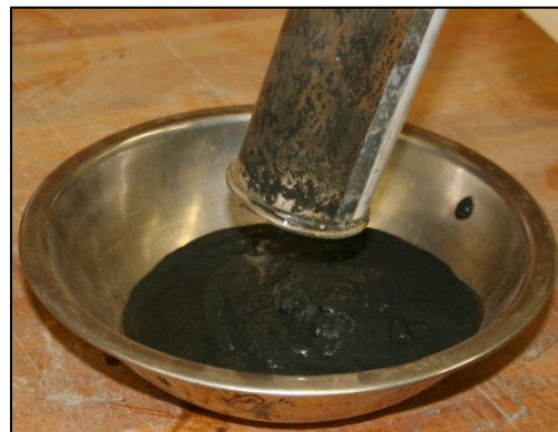
(f) Dewatered Slurry Removal
