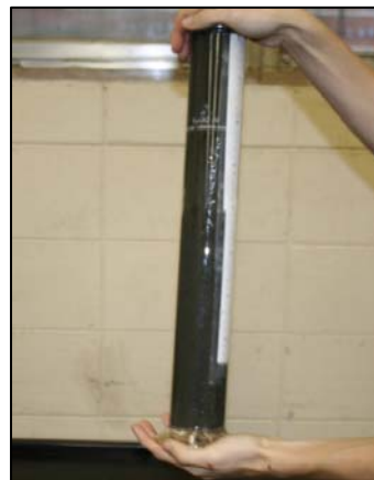
(d) Mixing of Soil Slurry and Polymer
