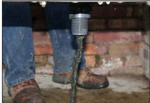
(b) Material Flowing from Geotextile Pillow
