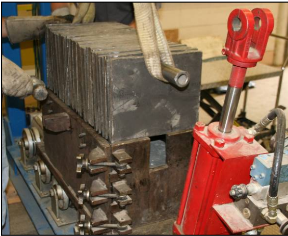
(c) Lowering Compaction Plates onto Mix
