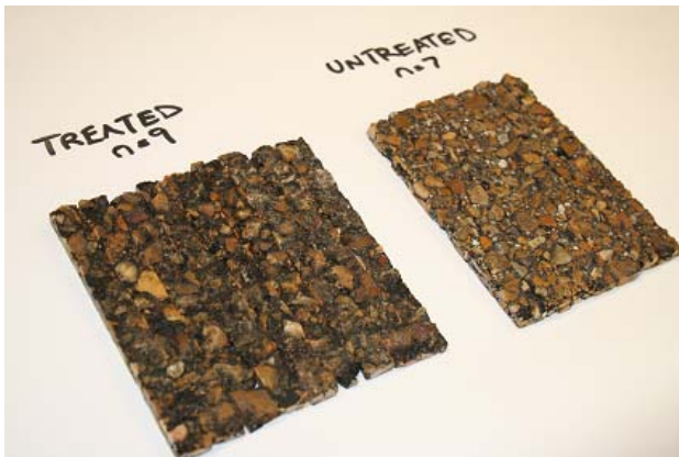
Figure 1. Photograph of BBR Test Specimens
