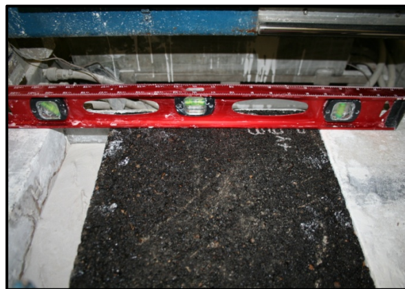
f) Checking Specimen Vertical Alignment
