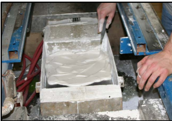
c) Spreading Plaster of Paris Mixture
