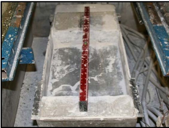
e) Leveling Front Block
