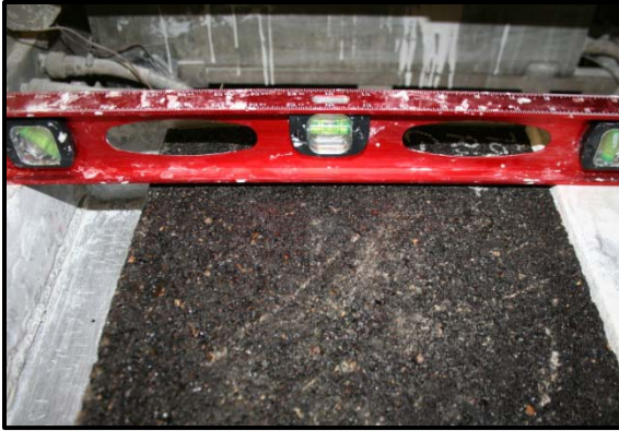
a) Dry Check of Specimen Height Alignment
