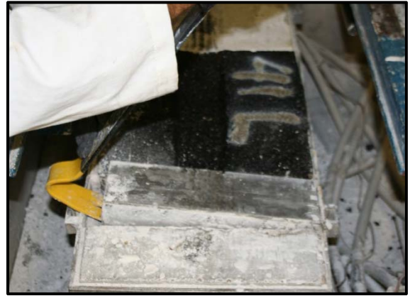
c) Removal of Spacer Block
