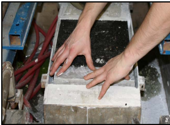
a) Placement of Spacer Block
