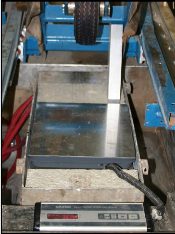
a) Contact Pressure Calibration Layout
