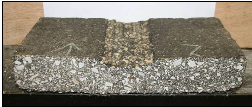
Figure 1. Example Slab from Original PURWheel
