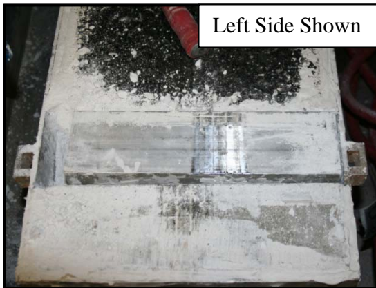
a) Spacer Block Ready for Removal
